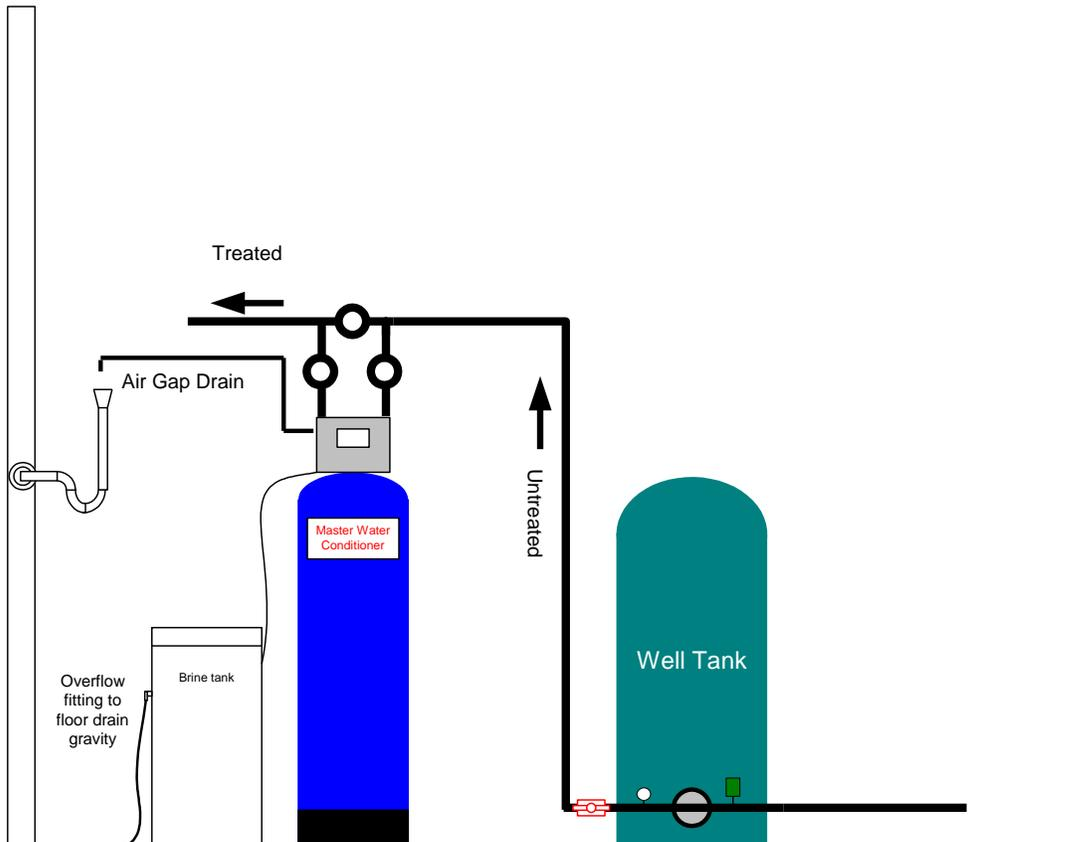
**NOTE:** All Master Water Conditioners must be installed after the well tank or water meter if its public water supply.
