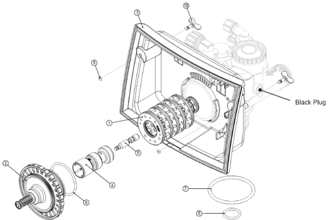
**Water Meter, Meter Plug and Mixing Valve**
