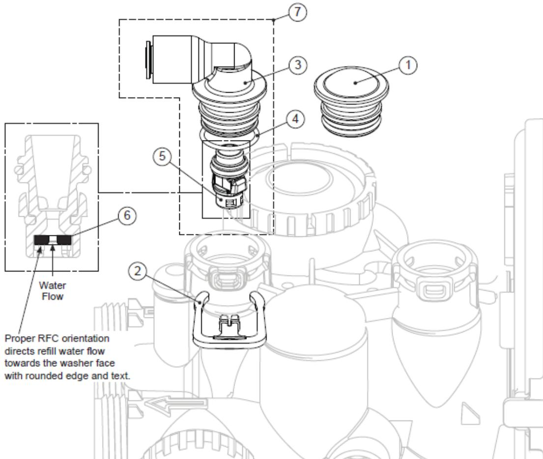
**Injector Cap, Injector Screen, Injector, Plug and O-Ring**
