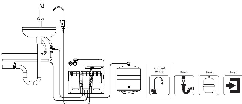
**Purified water.** Tube from the pure water outlet to the purified water faucet.
