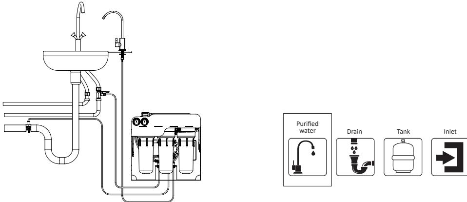
**Purified water.** Tube from pure water outlet to the purified water faucet.
