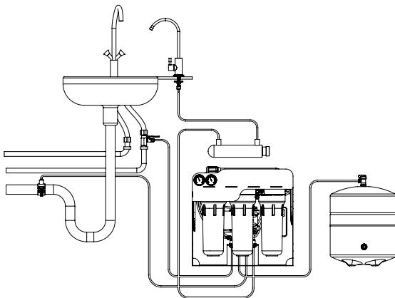
**Purified water.** Tube from the pure water outlet to the ultraviolet unit.
